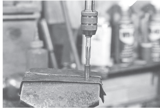
FIGURE 5 - Liner ONLY in padded vise jaws, chambering reamer in place.
