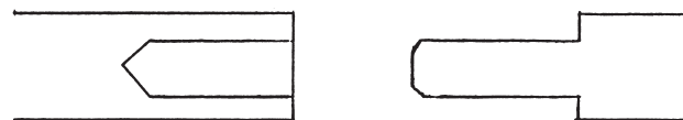
Short, Piloted Barrel Liner Drill - Center drill and drill 1"-1 1/4" deep - See instructions for suggested hole diameter.
