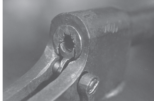
FIGURE 1 - Note severely eroded chamber. Barrel lining will eliminate this and restore accuracy. During examination, make as detailed a drawing as possible, showing location and details of extractor cuts, feed ramps, bullets, etc.
