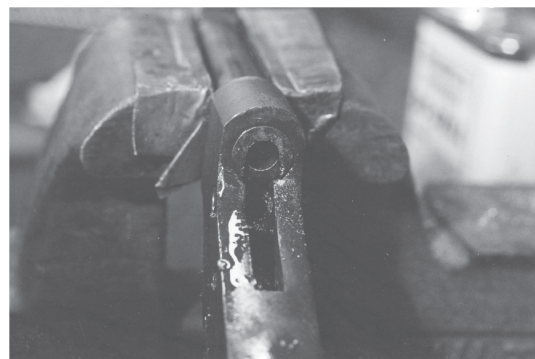
FIGURE 3 - Chamber end of drilled barrel. Note: Cutting oil must be thoroughly cleaned off before ACRAGLAS ® sing.
