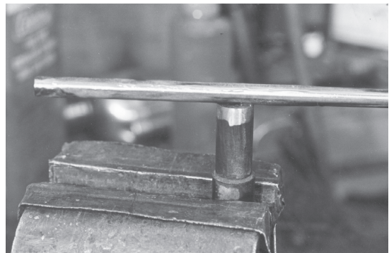
FIGURE 11 - Liner coated with ACRAGLAS, ready to install.
