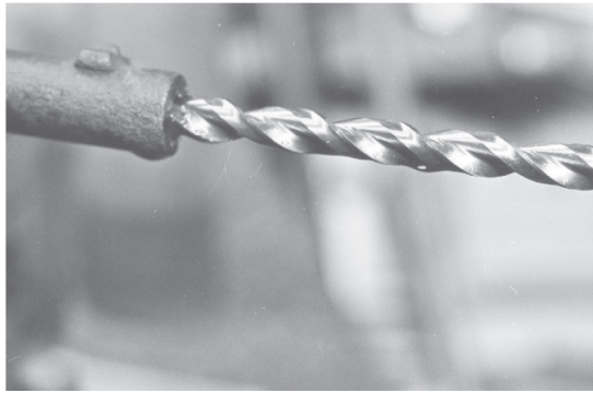
FIGURE 2A & 2B - Barrel is drilled SLOWLY with lots of oil, frequent chip removal and cleaning. Drill half of barrel length from each end with 1" overlap.
