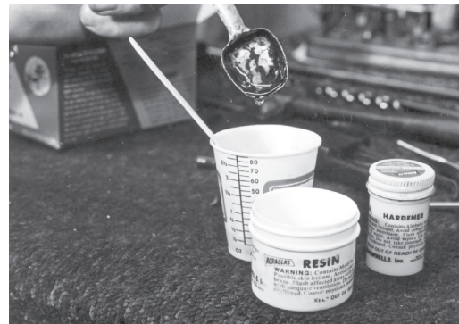
FIGURE 10 - ACRAGLAS kit comes with everything needed. Mix according to Instructions, but leave out the floc and walnut stain.
