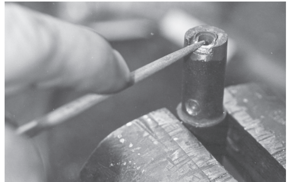
FIGURE 9 - Large extractor cutout requires bonding liner in barrel before making cutout.
