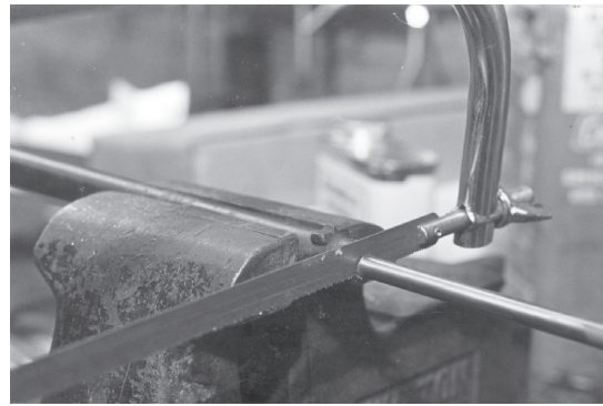
FIGURE 13A - Hacksaw excess liner off.
