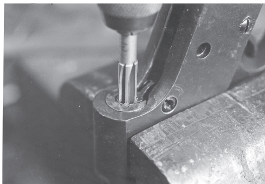
FIGURE 12 - Liner bonded, new extractor being fitted using chambering reamer to cut proper case body and rim clearance extractor.
