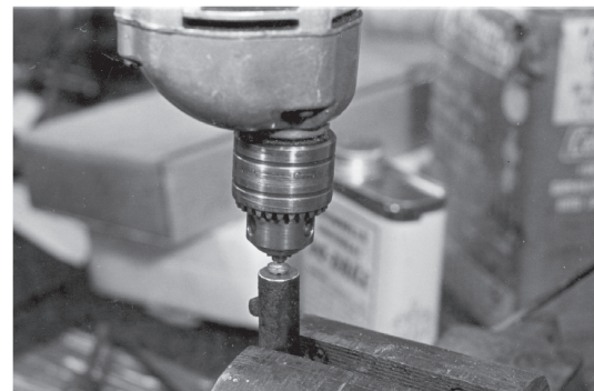
FIGURE 14 - Crowning the new liner using a round-headed brass bolt coated with fine grinding compound and mounted in an electric drill. Lightly bevel the inside edge of the new liner to blend with the original crown.
