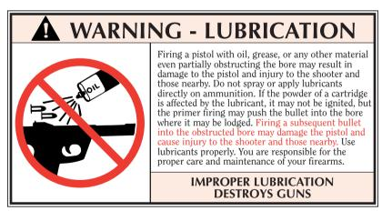
4. **NOTE:** Only a light application of oil is needed to provide adequate lubrication of moving parts and to prevent rust. Excess accumulations of oil tend to attract particles of dust and dirt and may congeal in cold weather, which can interfere with the safe and reliable function of the pistol.
