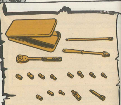
WRENCH SET, SOCKET: 1/4-in sq-drive, hex and 8 pt opngs, w/case.
