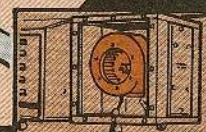
EXHAUST BLOWER — Blower switch ON, fails to exhaust.
