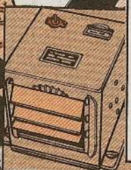
HEATERS — With switch on HEAT, fails to get warm airflow when operating temperature control; with switch on FAN, heating element stays on, fails to blow air; with switch OFF, fan continues to blow.
