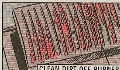
CLEAN DIRT OFF BURNER
