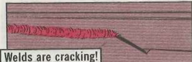
Welds are cracking!
