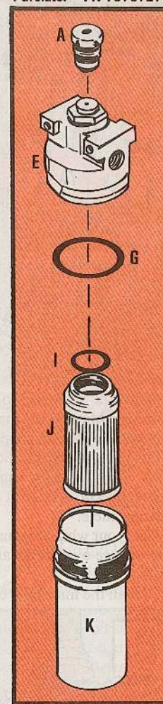
Hydraulic filter assembly- Purolator PN 7576727
