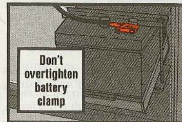
Clamp cable in place correctly
