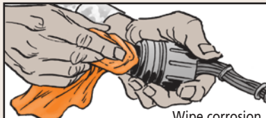
Wipe corrosion off connector with cheese cloth
