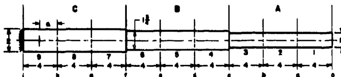
FIGURE 12. Gun Tube Showing Subdivisions.
