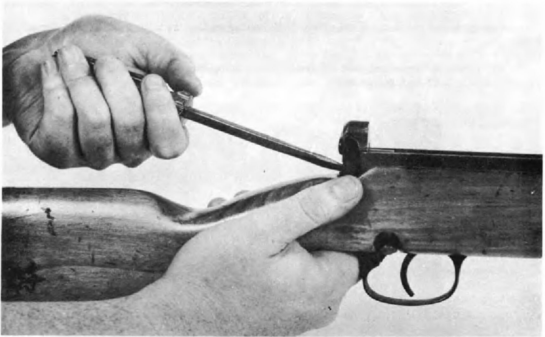
FIGURE 66. REMOVING TRIGGER MECHANISM (STEP 1).
