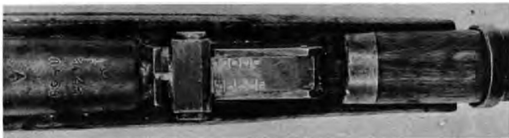
FIGURE 31. REAR RAMP SIGHT FOR CARBINE M1938.
