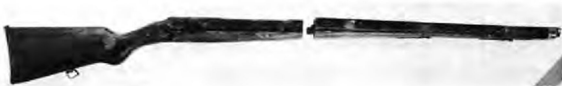
FIGURE 58. TWO-PIECE STOCK OF THE SEMIAUTOMATIC RIFLE M1938.
