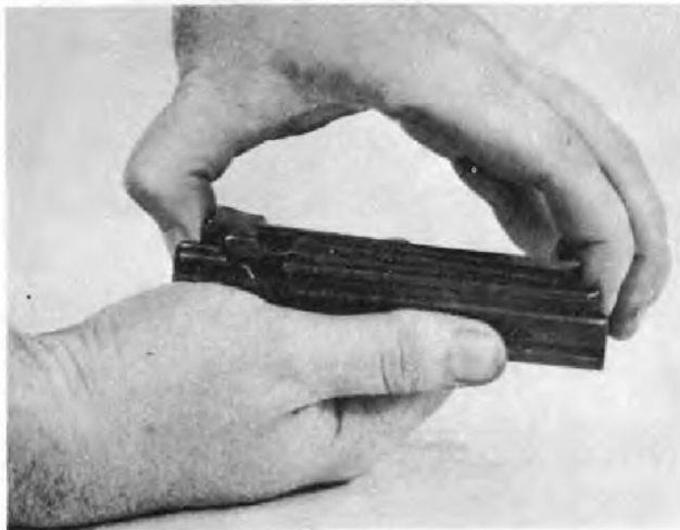
FIGURE 65. REMOVING BOLT FROM SLIDE.
