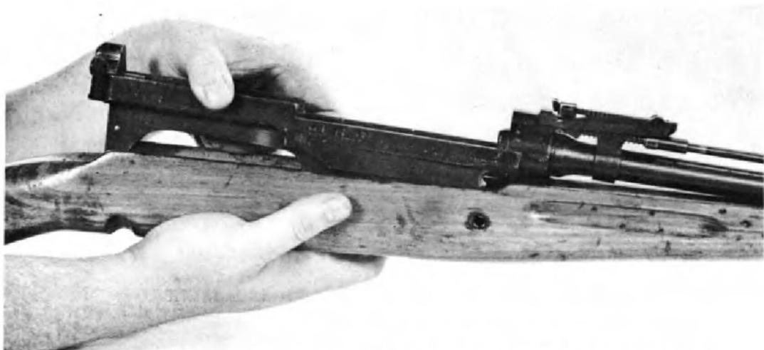
FIGURE 72. LIFTING THE RECEIVER AND BARREL OUT OF THE STOCK.
