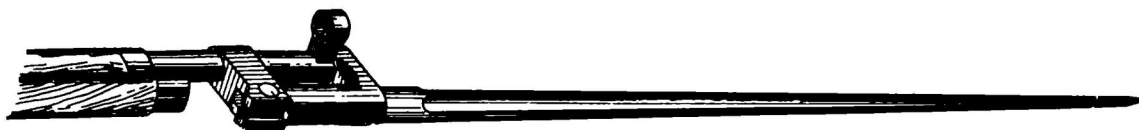
FIGURE 32. BAYONET FOR CARBINE M1944.
