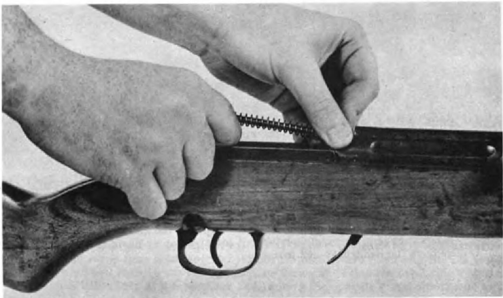
FIGURE 63. REMOVING DRIVING SPRING.
