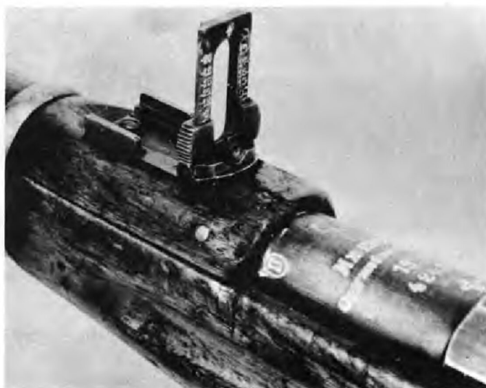
FIGURE 15. REAR SIGHT FOR CARBINE M1910.
