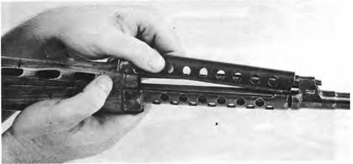
FIGURE 69. REMOVING THE TOP BARREL JACKET.
