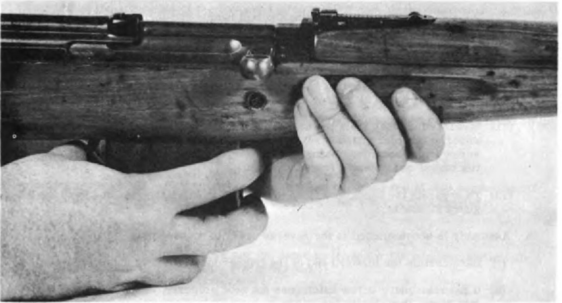
FIGURE 60. REMOVING MAGAZINE FROM TOKAREV RIFLE.
