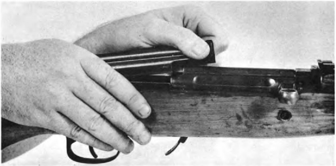
FIGURE 62. REMOVING BOLT COVER.
