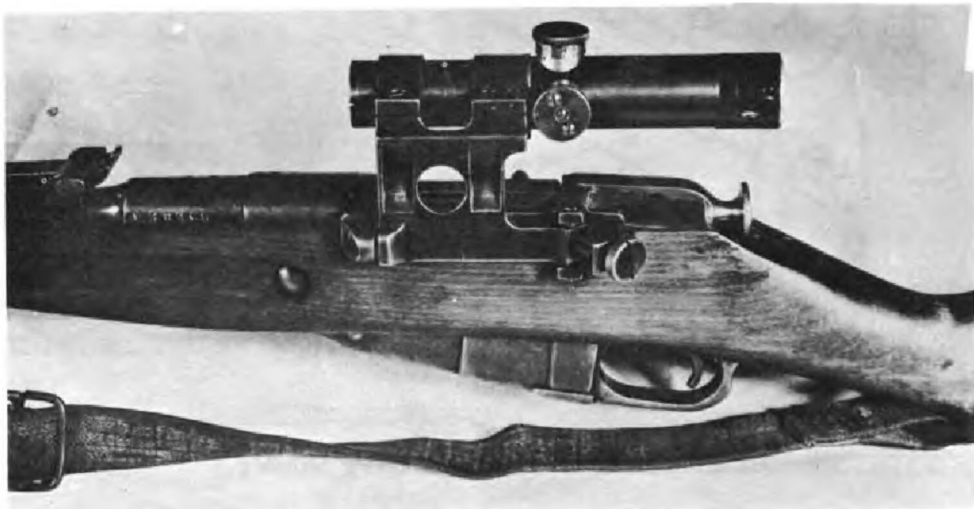
FIGURE 28. SNIPER RIFLE WITH PU TELESCOPE AND MOUNT (LEFT SIDE).
