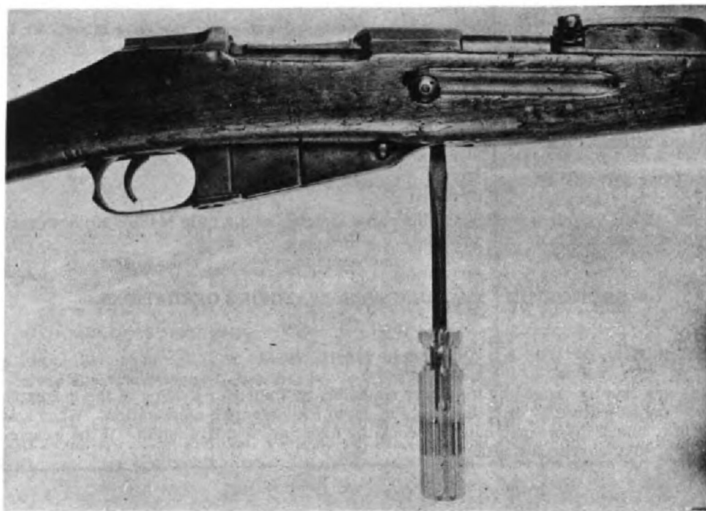
FIGURE 50. REMOVING THE FRONT TRIGGER GUARD SCREW.
