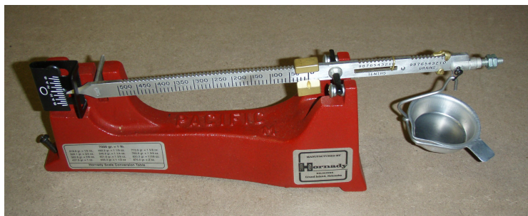
Figure 2.1: A Hornady mechanical beam scale for powder weighing. The graduated beam provides 0.1-grain resolution, and the magnetic damper (left) settles the beam quickly. Beam scales require no power source and never drift, making them an essential backup even on a modern bench. Photo: Arthurrh, CC BY-SA 3.0, via Wikimedia Commons.
