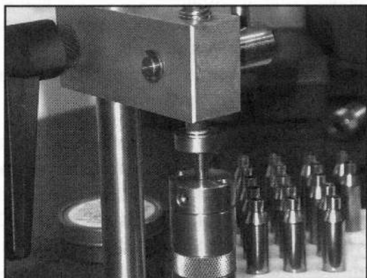
Arbor press pushing the sized case out of the die while depriming
